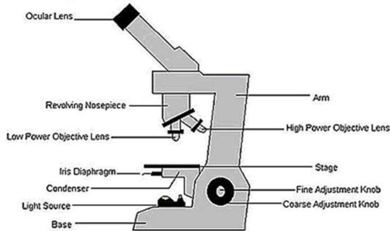
Parts of the Microscope
